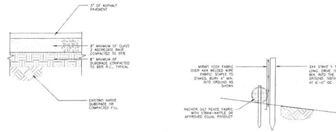
3 TYPICAL ASPHALT PAVEMENT SECTION C2
