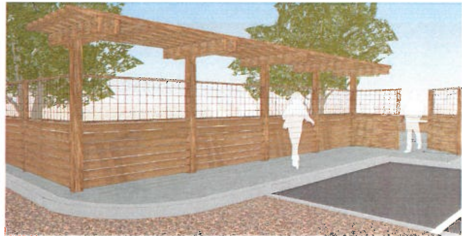
(V3) VIEW LOOKING WEST TOWARDS BACK PATIO FROM PARKING LOT HORIZONTAL AND HORIZONTAL SLAT TENDING WITH OVERHEAD TRELLIS AT PATIO ENTRANCE DOUBLE SLIDING GATE WITH 18" SIDE OPENING
