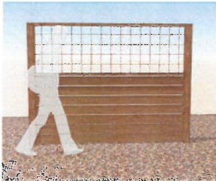
(F1) FENCE 1 - PATIO FENCE ENCLOSURE 6' TALL WITH 6' x 6' HOGWIRE PANELS AND HORIZONTAL REDWOOD SLATS
