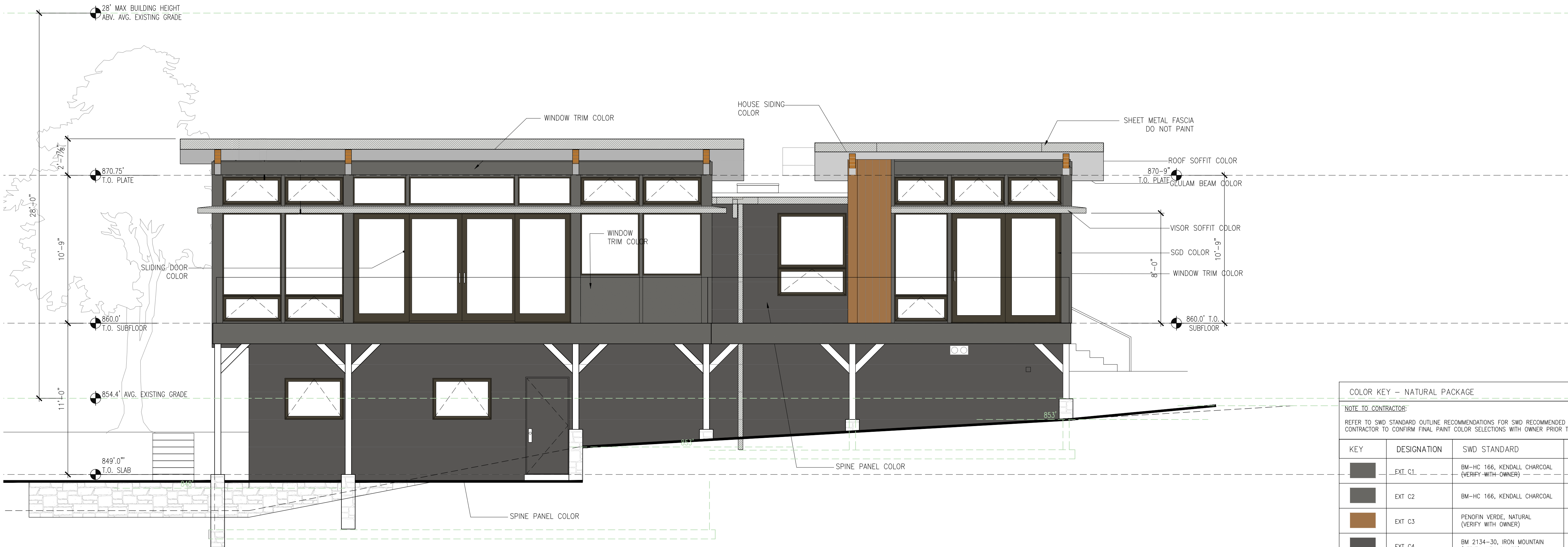
1 PAINT DIAGRAM - SOUTH ELEVATION 1/4"=1'-0"
