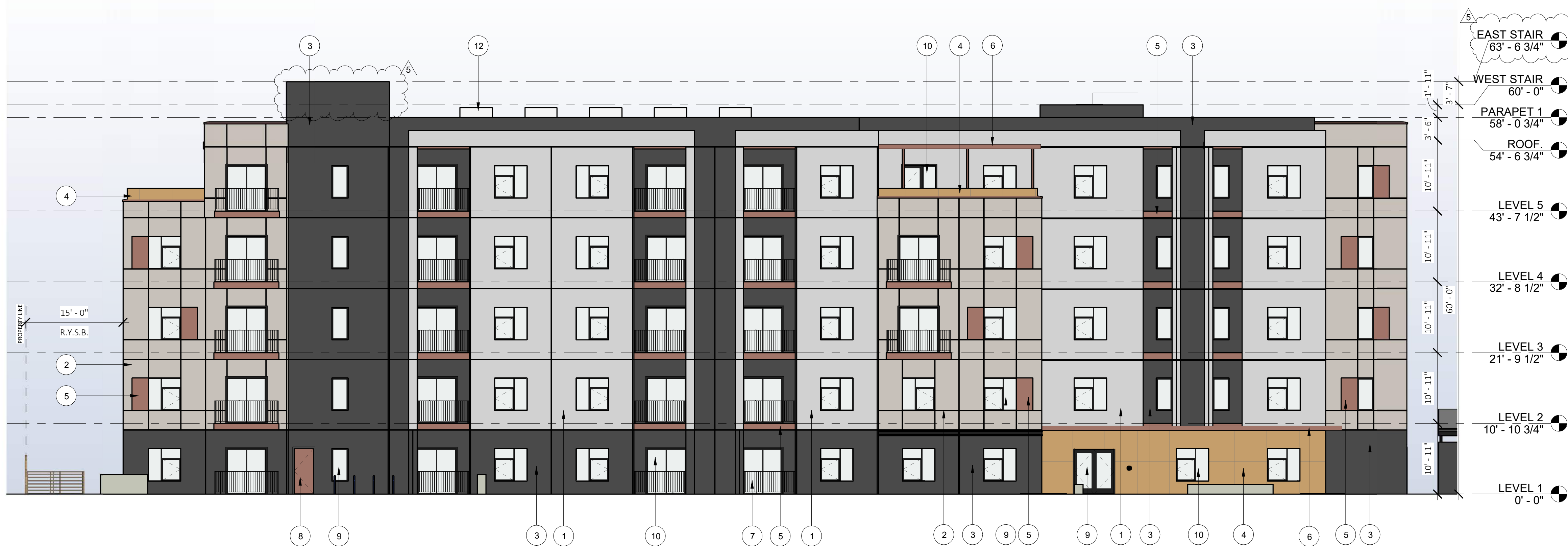
1 BUILDING ELEVATION - NORTH 1" = 10'-0"
