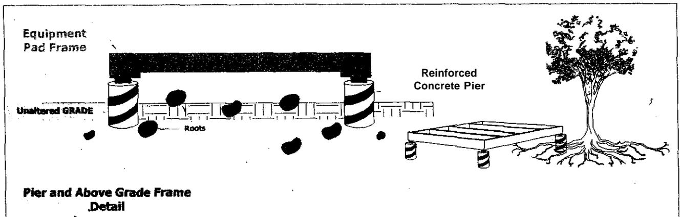
Piers will be placed at the corners of the 8 ft x 12 ft support **structure**. Grade beams will be placed above **natural** grade or constructed **without** disturbing native **soil**. This alternative method of construction will decrease the impacts of the pad **foundation**.
