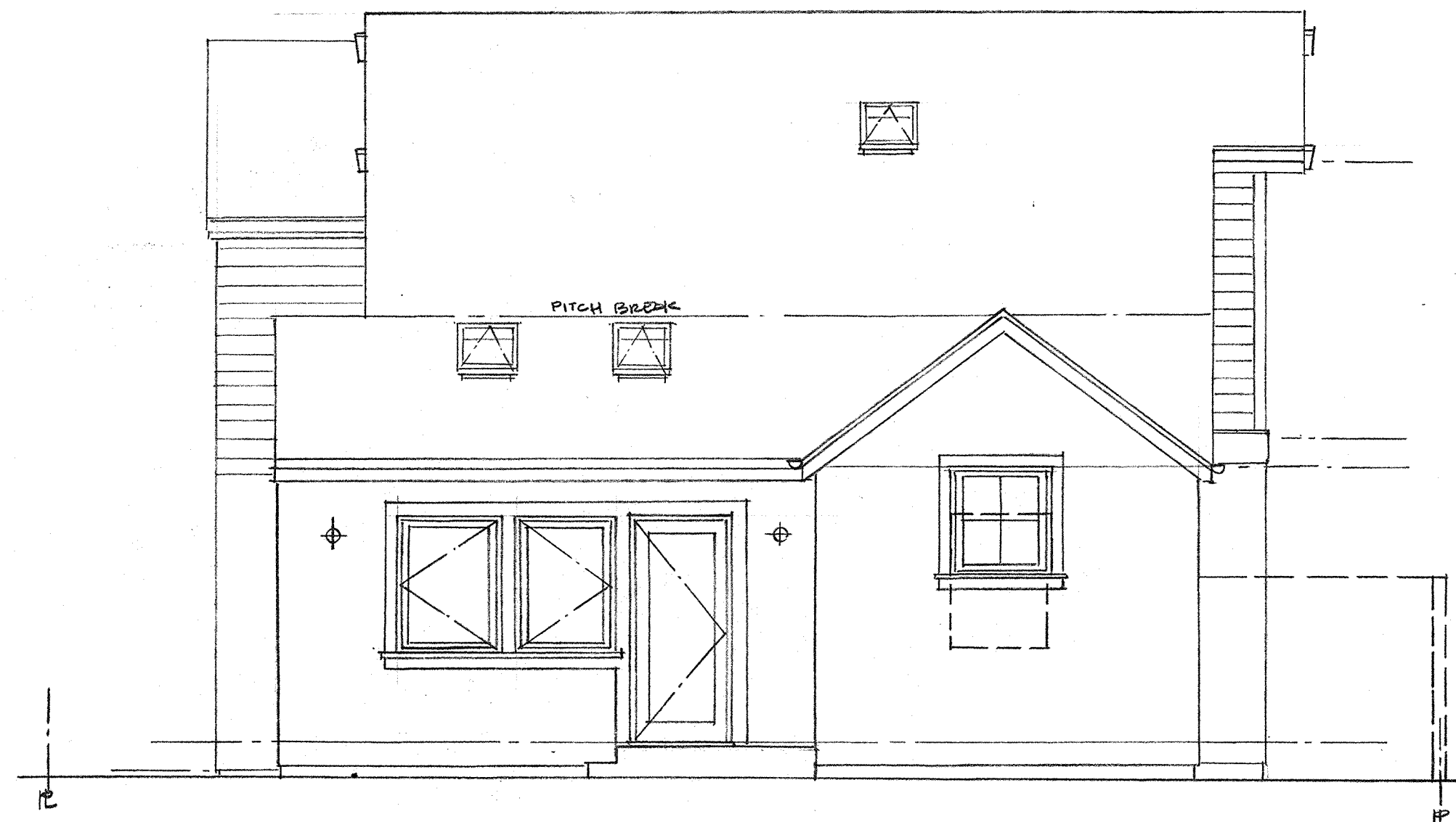
PROPOSED – WEST ELEVATION SCALE: 1/4" = 1'-0"
