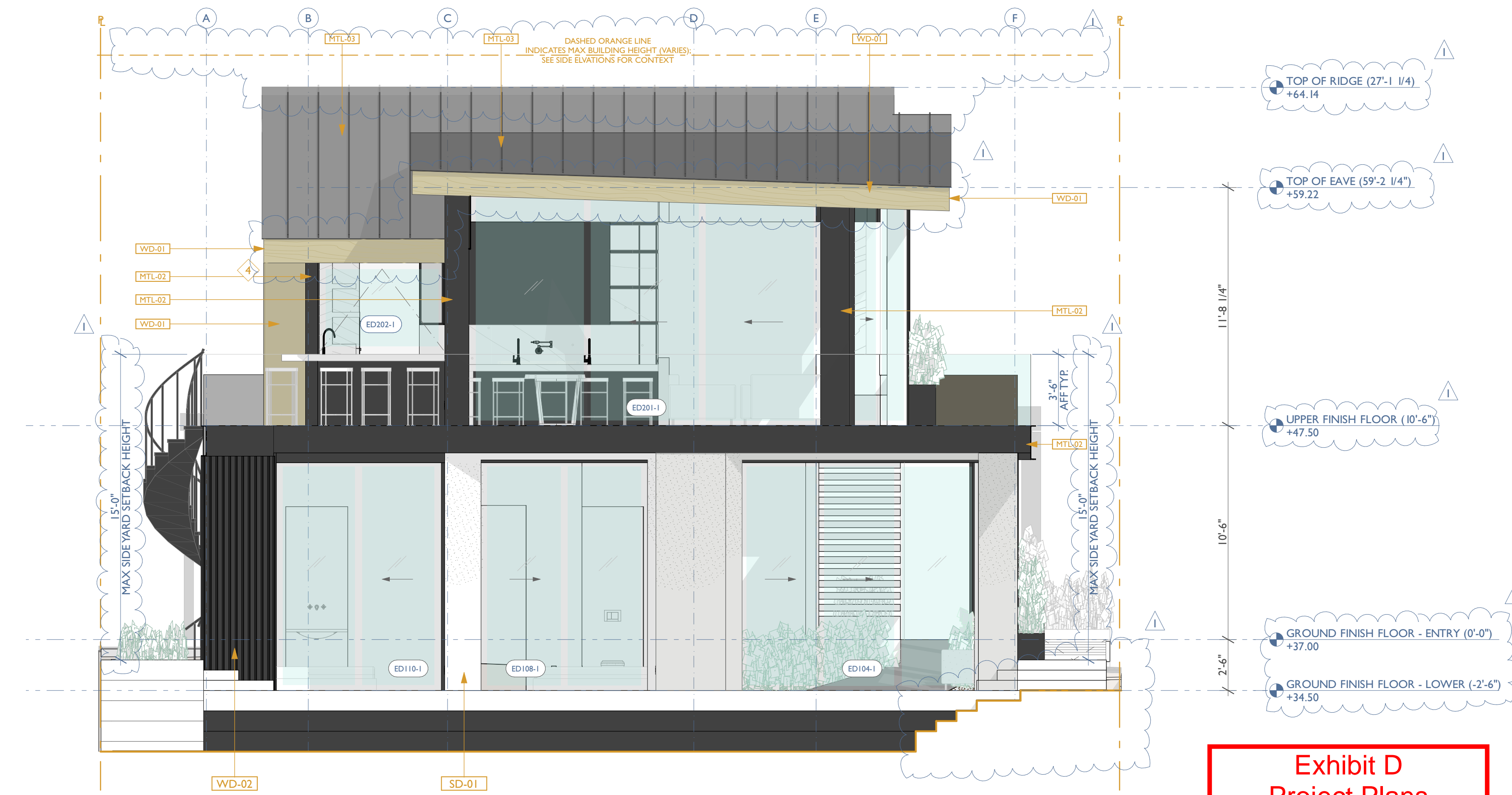
1 REAR EXTERIOR ELEVATION (northwest) SCALE: 1/4" = 1'-0"
