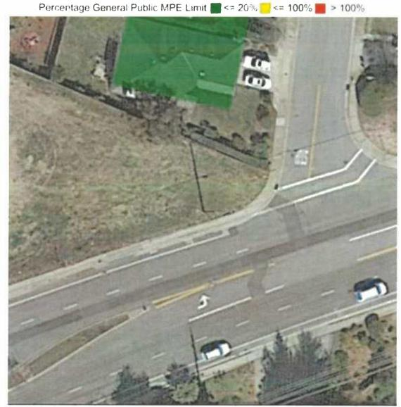
A 200 foot by 200 foot grid surrounding the site with the **general public MPE limit** calculated for accessible areas at roof level, approximately 20 feet above ground level, with all antennas operating. All accessible areas are within the general public limit. The maximum predicted power density in any accessible area is less than **1.0% of the general public MPE limit**.
