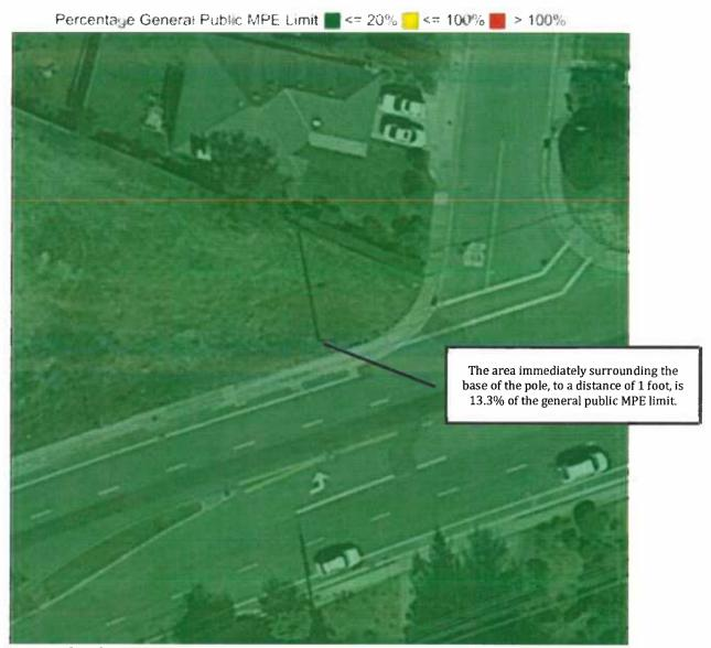
A 200 foot by 200 foot grid surrounding the site with the **general public MPE limit** calculated for ground level, with all antennas operating. All accessible areas are within the general public limit. The maximum predicted power density in any accessible area is **13.3% of the general public MPE limit**.
