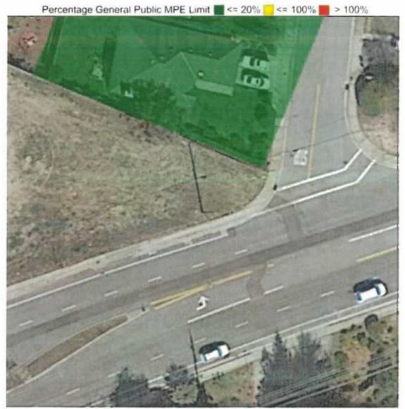
A 200 foot by 200 foot grid surrounding the site with the **general public MPE limit** calculated for ground level, with all antennas operating. All areas within the adjacent property are within the general public limit. The maximum predicted power density in any area is less than 1.0% of the general public MPE limit.
